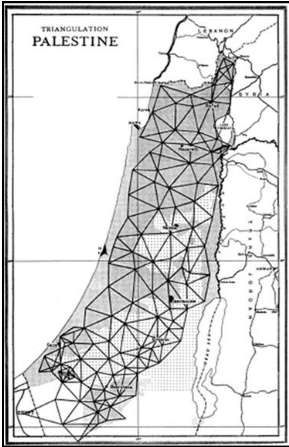
Figure (7): The Major Triangulation system in Palestine in 1946 (Gavish, 2004, conducted by author).
